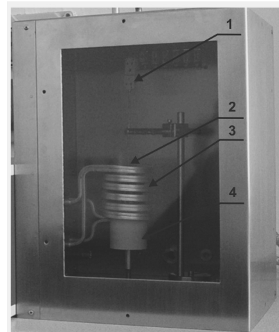
Fig. 1. Working chamber of the UMSA device: 1 – thermocouple, 2 – tested sample, 3 – induction coil, 4 – ceramic isolation
