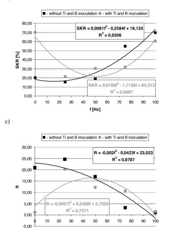
Fig. 5. Influence of frequency (f) of supply current feeding induction coil, which generates electromagnetic field on selected refinement parameters of structure of pure Al ingot
