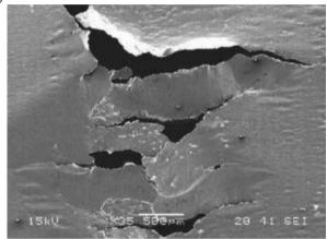
Fig. 1. Phase  $TiB_2$  in structure of pure Al (a) and produced in result from its present crack in sheet (foil) during rolling [12]
