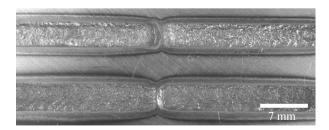
Fig. 18. Face view after laser alloying with vanadium carbide, 32CrMoV12-28 steel, laser power of 1.2-2.3 kW
