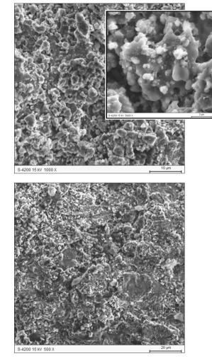
Fig. 13. Morphology of NiAl(Cr)-Al<sub>2</sub>O<sub>3</sub> coating a) –after 48 h exposure time, b) 500 h exposure time
