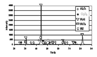
Fig. 10. X-ray diffraction of corrosion products after tests at a temperature of 600°C and in the period of 48 hours
