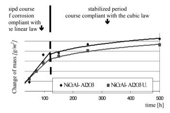
Fig. 12. Changes of the samples' mass in time function at a temperature of  $600^{\circ}$ C with marked periods which are characterized by the linear and cubic corrosion law
