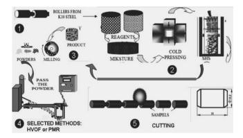
Fig. 3. Five stages of preparing the samples for the corrosion test
