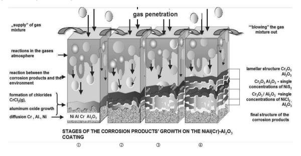
Fig. 16. Suggested mechanism of coating's corrosion: Growth of corrosion products on the surface of NiAl(Cr)-Al<sub>2</sub>O coating during the corrosion process:  $\mathbb{O}$ the course of reaction connected with chlorides' formation (in gas and molten form),  $\mathbb{O}$ slow growth of aluminium and chromium oxide  $\mathbb{O}$ - $\mathbb{O}$  reactions connected with the formation of nickel chlorides, sulphides and subsequent oxide layers
