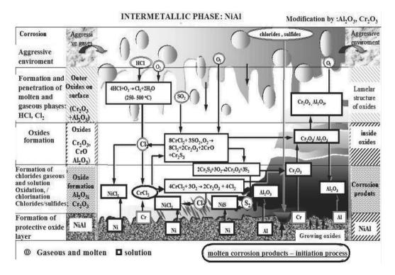
Fig. 17. The corrosion mechanism of NiAl(Cr)-Al<sub>2</sub>O<sub>3</sub> coatings in aggressive environments: N<sub>2</sub>+9%O<sub>2</sub>+0.2%HCl+0.08%SO<sub>2</sub>
