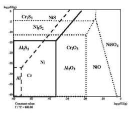
Fig. 8. Overlapped Ni-O-S, Cr-O-S and Al-O-S phases stability diagrams for temperature of 927 K
