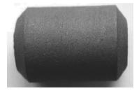
Fig. 6. A view of the NiAl(Cr) – Al<sub>2</sub>O<sub>3</sub> coating surface, magn. 2x
