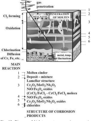
Fig. 15. Diagram of high-temperature corrosion course in an environment containing a mixture of gases: HCl;  $O_2$  and  $SO_2$  [4]
