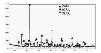
Fig. 2. Composition of NiAl(Cr) –  $Al_2O_3$  powder after SHS synthesis
