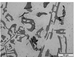
Fig. 5. a), b) Microstructure of ACAlSi9Cu casting alloy
