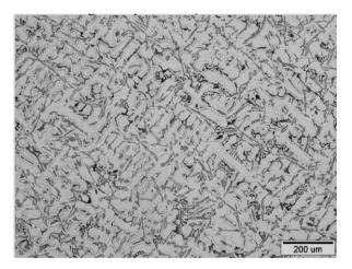
Fig. 7. Microstructure of ACAlSi9Cu4 casting alloy
