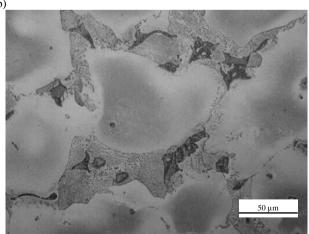
Fig. 2. a), b) Microstructure of MCMgAl6Zn1 magnesium alloys in as-cast state
