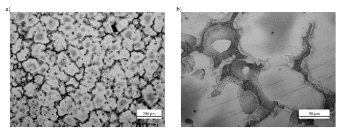
Fig. 3. a), b) Microstructure of MCMgAl9Zn1 magnesium alloys in as-cast state
