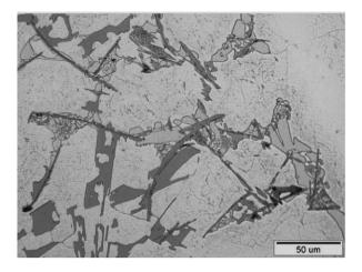
Fig. 6. Microstructure of ACAlSi9Cu4 casting alloy
