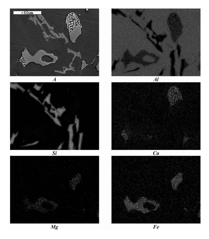
Fig. 8. The area analysis of chemical elements alloy ACAISi9Cu4: image of secondary electrons (A) and maps of elements' distribution
