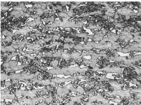
Fig. 2. Multiphase structures with various fractions of retained austenite for the thermo-mechanically processed specimens, isothermally held in a bainitic transformation temperature of 250^\circ\text{C} (a), 300^\circ\text{C} (b), 350^\circ\text{C} (c), 400^\circ\text{C} (e), 450^\circ\text{C} (g), 500^\circ\text{C} (h) and selected binary maps showing regions corresponding to retained austenite for the specimens held at 350^\circ\text{C} (d) and 400^\circ\text{C} (f)
