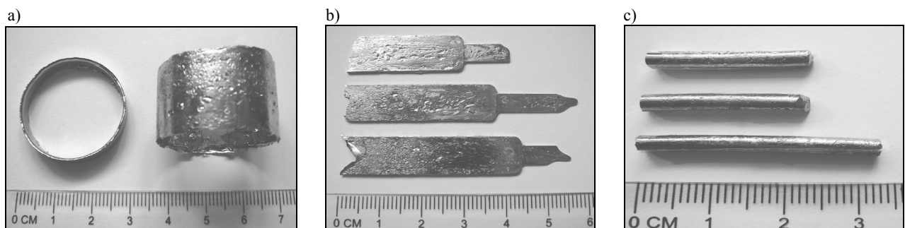
Fig. 5. Outer morphology of cast glassy \text{Fe}_{43}\text{Co}_{14}\text{Ni}_{14}\text{B}_{20}\text{Si}_5\text{Nb}_4 alloy samples in form of: a) rings, b) plates, c) rods
