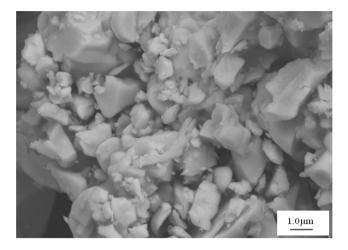
Fig. 5 Mixture of WC powder (97%), Co powder (3%) after 8 hours of milling in the ball mill
