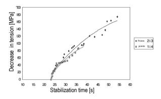
Fig. 9. The dependence of stress drop on the temperature stabilization time for measuring points 2, 3 and 1,4
