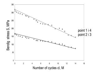
Fig. 7. Dependence of bending stress at the measuring points 2, 3 and 1, 4 on the number of fatigue cycles
