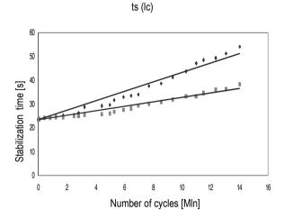
Fig. 8. Dependence of temperature time stabilization versus the number of fatigue cycles for measuring points 2, 3 and 1, 4
