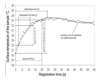
Fig. 4. The course of temperature changes during thermographic measurement
