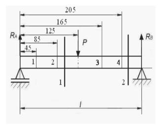
Fig. 2. Diagram of the distribution of forces and reactions acting during deformation of the sample in the fatigue machine and the distribution of measurement points: 1,2,3 and 4
