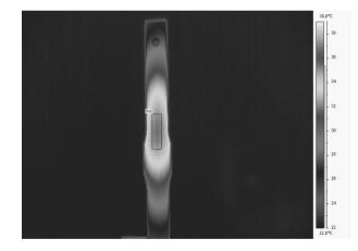
Fig. 5. Example thermogram for the samples subjected to fatigue tests at 10 million cycles (the temperature was read from inside the selected rectangular area)
