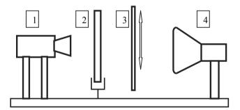
Fig. 3. Schematic draw of thermovision research stand. 1 - thermovision camera, 2 - sample, 3 - removable shield, 4 - infrared radiator
