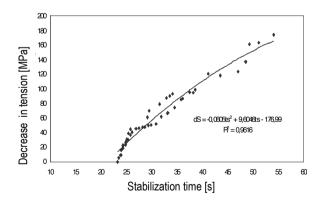
Fig. 10. The relationship between the drop in the bending tension found out in fatigue procedure and the temperature stabilization time specified in thermographic investigations
