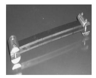
Fig. 1. A set of samples from the polyethylene spacer for fatigue tests
