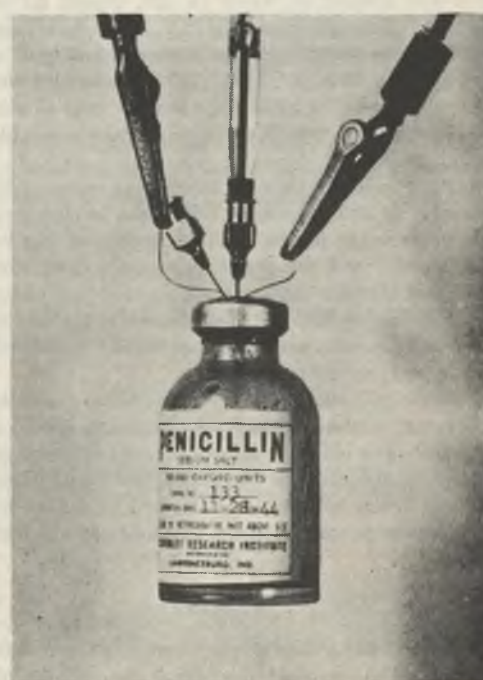
Figure 2. Penicillin Bottle Used as Titrating Vessel
