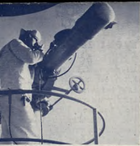
A seaman manning a 2½ meter Range Finder reports range continuously during action.—U. S. Navy Photo.
