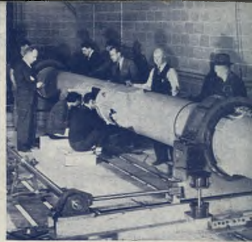
Test chamber duplicates the continuous vibration of the ship and the shock of a broadside of heavy guns.
