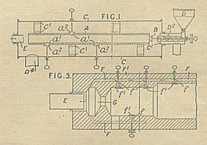
(Fig. 3) ducts, F, are formed in the retort lining,  $F^1$ , and the heating gases, throttled by a constriction, G, are forced along the ducts and through the openings, f, controlled by valves,  $f^1$ . The retort may be inclined or vertical, or may be rotary, and when treating strongly caking coals these may be passed through a heating and a cooling zone before being further heated, thereby avoiding clogging of the retort.
