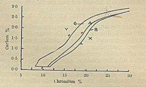
to the co-ordinates of any point within an area A. bounded by lines, a, b, c, d on the graph are hardened and rendered immune to food acids by heating them to 24—300° above their upper transformation point and cooling rapidly. C. A. KING.
