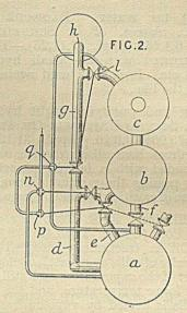
is connected to the pipe, h, through a valve, l, to enable water-gas to be re-circulated through the plant. Steam is supplied through valves, n, p, q, to the required parts of the plant, and the valves are coupled as shown by the full thick lines; the broken lines indicate interlocking means between the valves. S. PEXTON.
