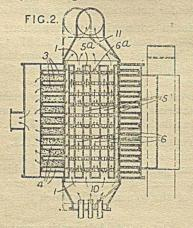
compartments used alternately for heating (4) and for containing the material (3). The annuli for heating are provided with radial guiding partitions, alternate sides of which are in communication with passages, 5, for heating gases, or 6 for exhaust gases in the central part of the furnace. The passages 5 are closed at one end of the furnace and the passages 6 at the other. B. M. VENABLES.
