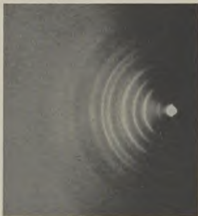
Fig. 2—Electron diffraction pattern obtained by the reflection method from finely pulverized aluminum alpha-monohydrate ( \text{Al}_2\text{O}_3 \cdot \text{H}_2\text{O} ).
