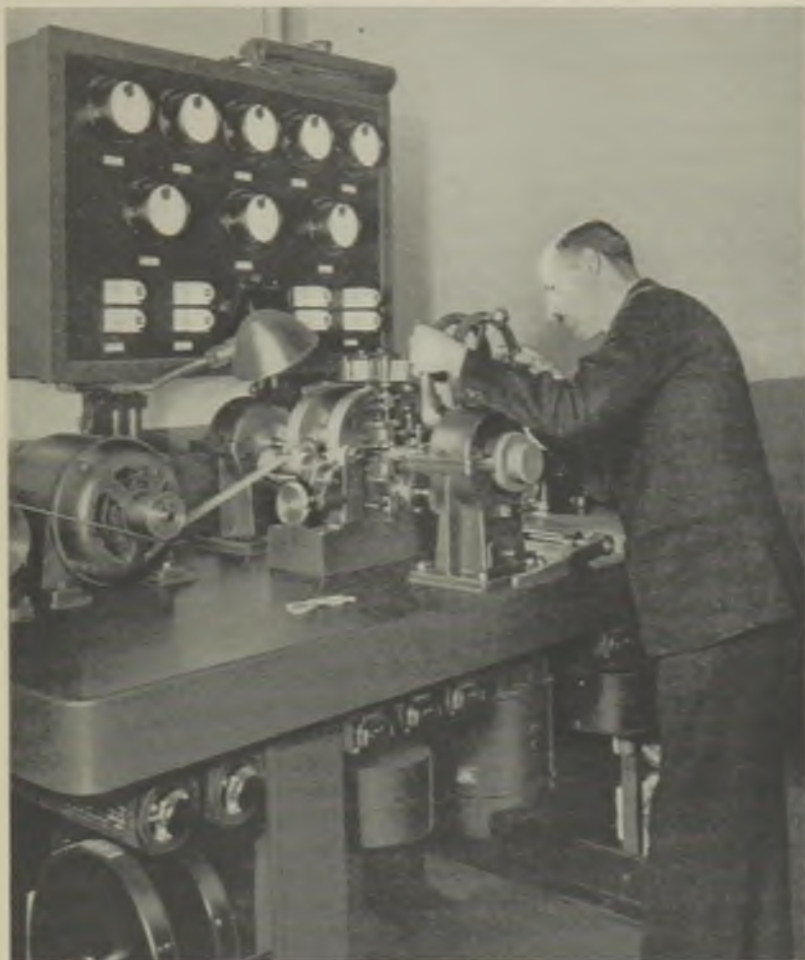
Fig. 6—Twenty roll cold-reduction mill for producing thin sheet materials for experimental studies.
