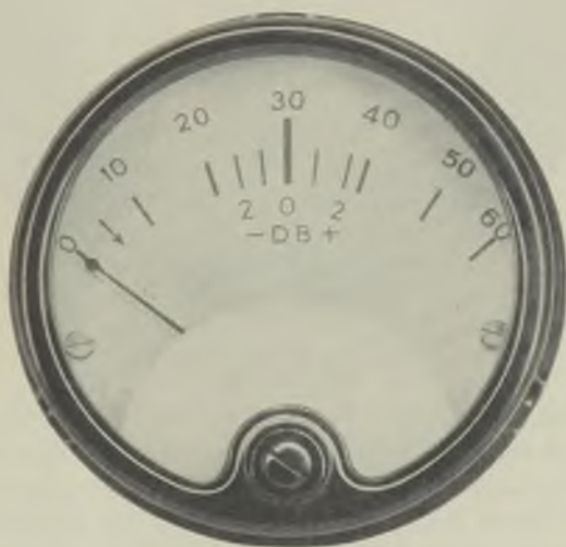
Fig. 12—Scale on 203C volume indicator.
