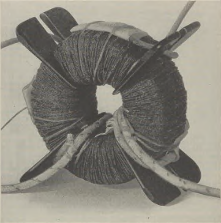
Fig. 7—Toroidal inductance coil used in crystal channel filter, shown before potting.
