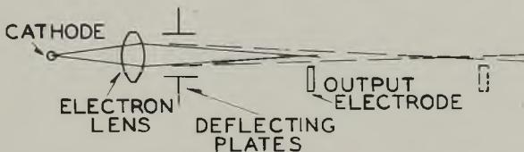
Fig. 4—Amplifying tube making use of electron deflection.
