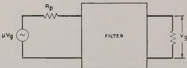
Fig. 12.17—Generalized oscillator circuit in the form of a filter network
