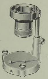
This improved model is provided with an integral protective skirt to the orifice. The base is precision machined, is removable from the body and can be interchanged with other bases having different orifice sizes. A ball valve is supplied for use in closing the orifice during filling.
