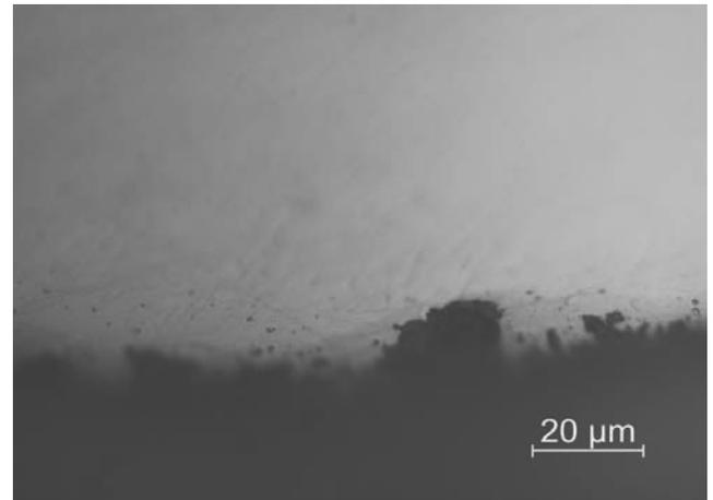
Fig. 4. Micropores and corrosion pits on a specimen surface after electrochemical investigations in the 0.5N NaCl
