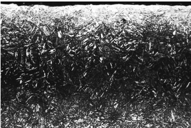
Fig. 27. Microstructure of plasma nitrided layer. Sample 34A2. Compact nitride and diffusion zones. Nital etching
