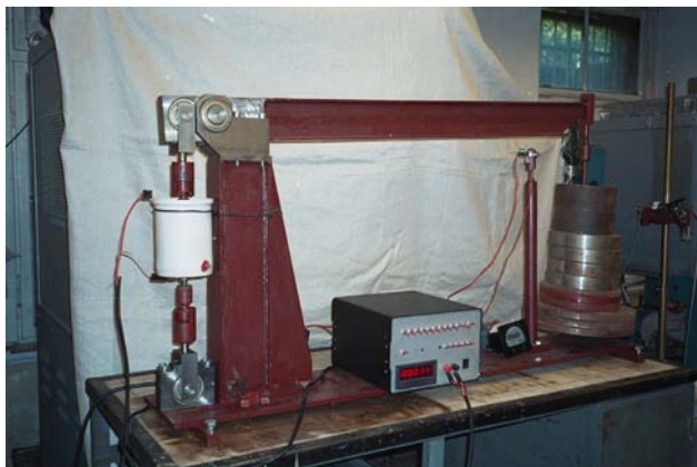
Fig. 18. View of the lever machine with the environmental cell
