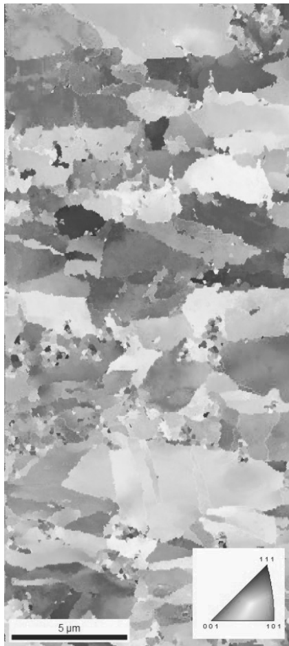
Fig. 28. Inverse Pole Figure (IPF) map after CRCS process of annealed sample strip
