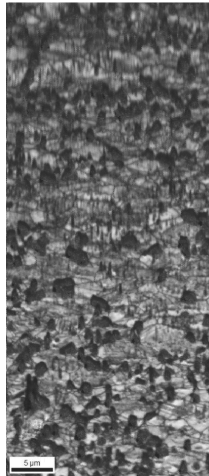
Fig. 26. Quality image map (IQ map) after CRCS processing of annealed sample strip
