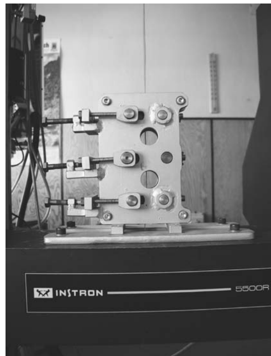
Fig. 8. CRCS rolling set installed in testing machine
