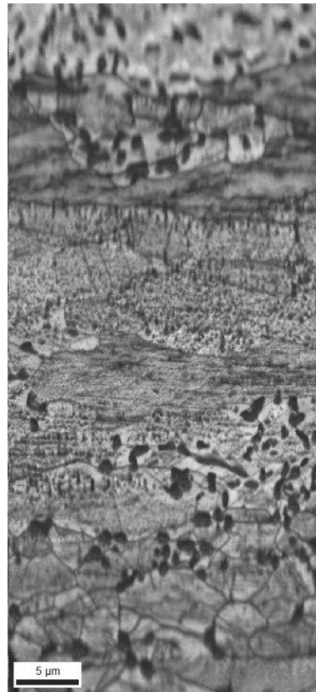
Fig. 22. Image quality map (IQ map) of annealed sample strip
