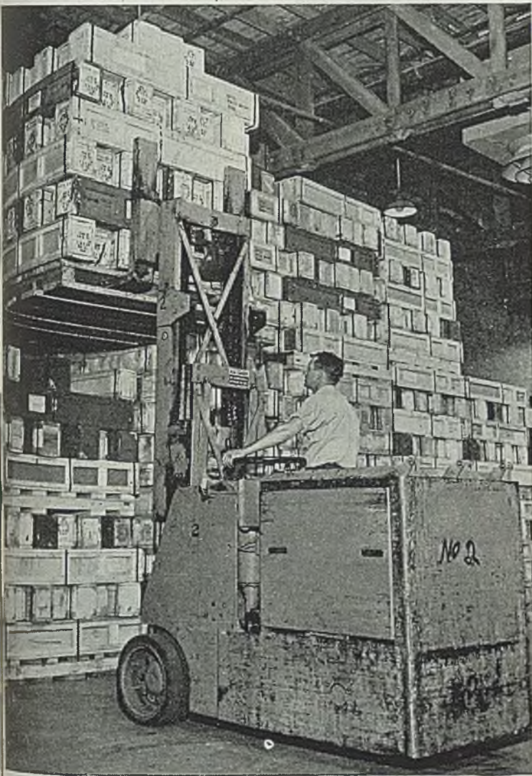
Tiering of materials to the ceiling permits maximum utilization of storage space. This is a stop-and-go handling job in which battery trucks excel because of their inherent flexibility and dependable operation.
