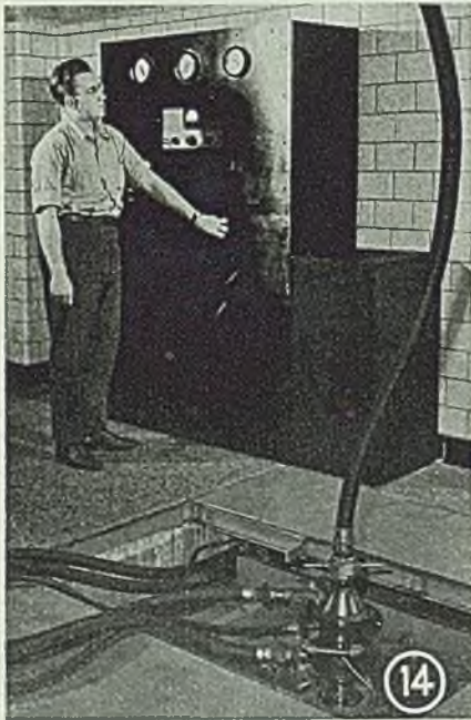
Fig. 14—View of Alcoa whirl pit with special air turbine that revolves specimens at speeds up to 60,000 rpm. Work is suspended from turbine shaft. Control panel in background
