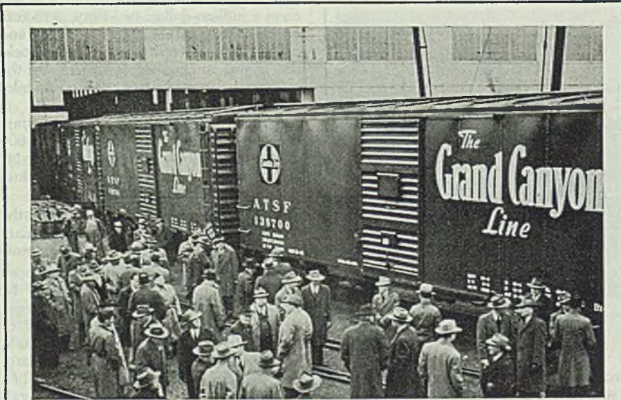
POSTWAR BOX CARS: First new standard steel box cars built by Mt. Vernon Car Mfg. Co., a division of H. K. Porter Co. Inc., are rolling from assembly lines at Mt. Vernon, Ill., where an order for 500 is being filled for the Atchison, Topeka & Santa Fe. Steel-sheathed and wood-lined, the cars are 40½ feet long, have capacity of 3966 cubic feet
