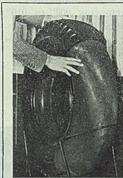
WIRE CORD TIRE: Four plies of medium carbon steel, hard drawn wire replace 10 plies of rayon cord in this tire developed by Firestone Tire & Rubber Co., Akron, for heavy-duty truck and bus use. Individual wire filaments are 0.0058-in. in diameter, and usual construction is 7x3—three filaments twisted together to form a strand and seven strands twisted to form a cable. Tests indicate 200 per cent greater strength than rayon, and tire runs about 30° cooler because of thinness due to high cord strength and quicker dissipation of heat
