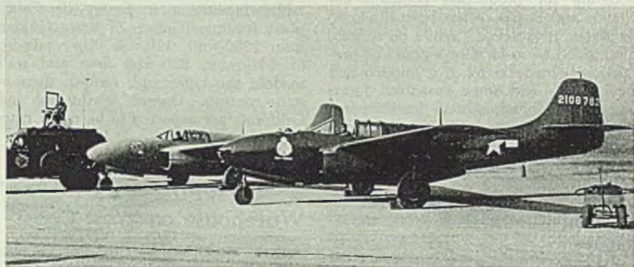
Three physical components of the remote plane control project developed by Air Technical Service Command and Bell Aircraft Corp. are shown here. Left to right are a panel truck which operates the controlled or robot plane and incorporates telemetering and television equipment for the observation and recording of flight research data; the robot plane and the "mother" plane. Both aircraft are P-59 Airacomet
