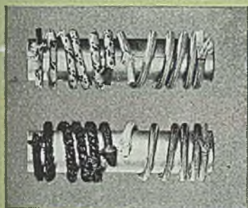
Cable insulated with Dow Corning Silicone rubber (at right) shows no change after one hour at 280° C., in contrast with organic rubber, which has melted and frayed freely through the braid.
