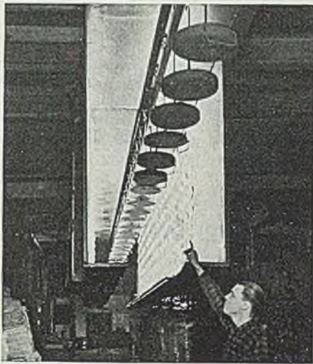
Below: Same parts going through one of the Japan Company infra-red ovens.
