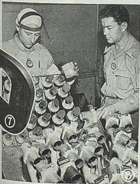
Fig. 7—Tooling method used to locate the tube bevel in relation to the flange hole pattern during a light press fit assembly operation
