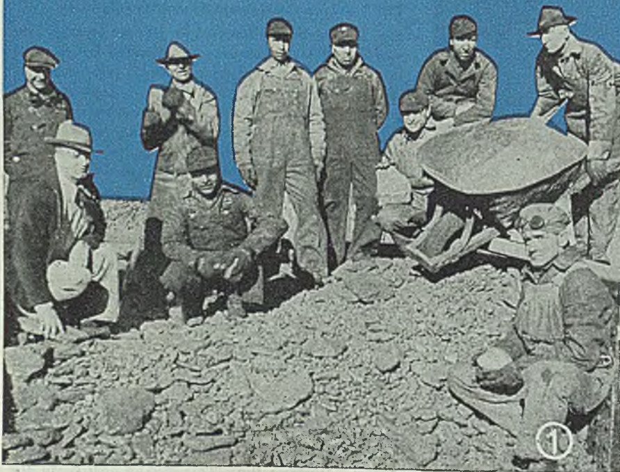
Fig. 1—Sponge iron nodules which were shipped to nearby steel plant
