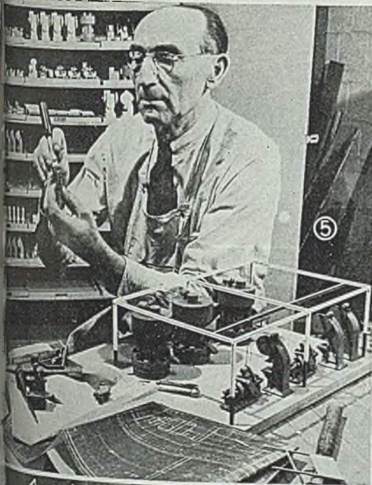
Fig. 7—Complete model layout of small plant and equipment, exact down to the smallest detail such as stairways, inspection benches and structural columns. For further study it is possible to place models of workmen at various machines
