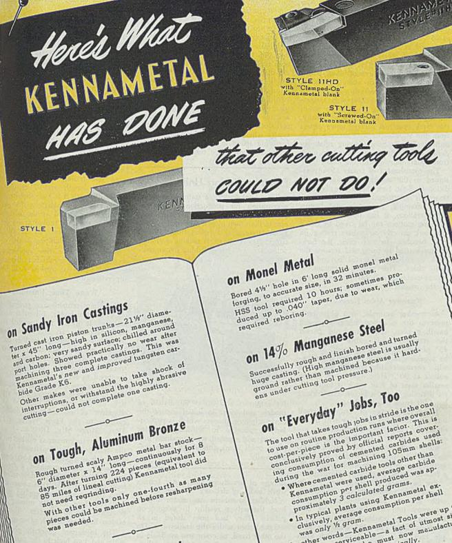
on Chrome Nickel Steel Rough turned very scaly chrome nickel forging -2' diameter x 10' long — in 30% less time, and with triple the tool life obtained from other tools, which could not stand up under the and with triple the tool life optained from other tools, which could not stand up under the plunge cut through scale.
