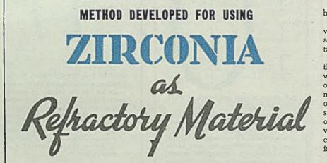
THE structural disintegration of refractory shapes made from zirconia can be eliminated by the addition of certain oxides that "stabilize" the crystal form of the material, and by special heat treatment, according to R. F. Geller, National Bureau of Standards, Washington, who has been working on this problem.
