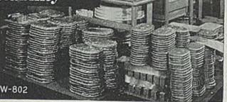
This picture clearly demonstrates the adaptability of the Blanchard. Here are a variety of pieces of cast iron, steel, and bronze ready to be ground on the No. 18 Blanchard Surface Grinder. Most of the pieces are to be ground on two sides, the usual limits being  $\pm .0005^{"}$  and the amount of stock removed from .015" to .020" per surface.
