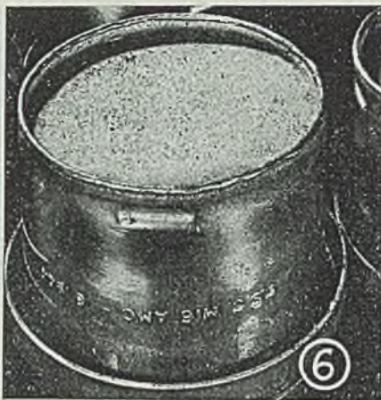
Fig. 6—Finished edge weld on bottom end. Note crimping which holds flanged bottom cap in position for welding
