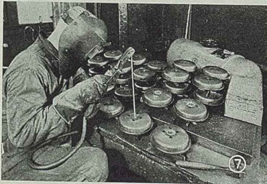
Fig. 7—Making plug welds on removable top caps. When clamped in place the cap keeps the powder dry, but can be removed in an instant
