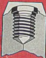
1. Drill counter-bore and top
