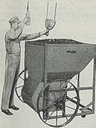
This bucket is \frac{1}{4} yard size and carries \frac{1}{2} ton of coal. It is used as shown below.
