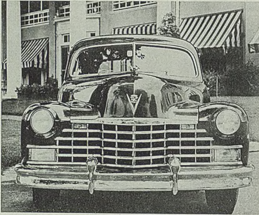
Built-in fog lights below main headlamps are a feature of the 1946 Cadillac front end styling. Bumpers have been strengthened and increased in size, while the chrome plated radiator grille has been "opened up" to permit easier cleaning and give better air intake
