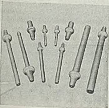
Above: —Group of Forged, Rough Turned and Bored Rings Weighing About 200 Pounds Each. Below: —Forged-to-Shape, Swaged, Sawed, Centered, Straightened, and Shot Blasted Milling Machine Arbors. V
