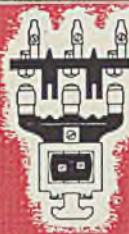
Switch open — plunger down — contacts open
