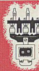
Switch closed — plunger up — contacts closed
