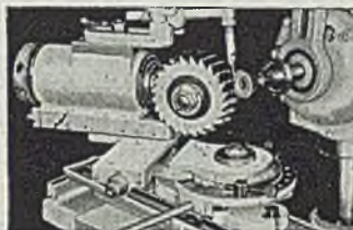
Grinding radius on 4" Milling Cutter
