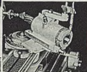
Grinding radius on Spiral End Mill
