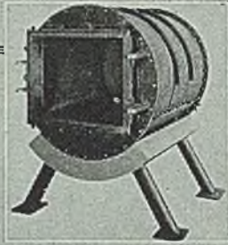
3000 lb. Electro Processing Oven of 1/2" steel plate (56" long x 36" inside dia meter) shown with rock wool jacket removed. . . fabricated by Brandt for a large cork board plant.
