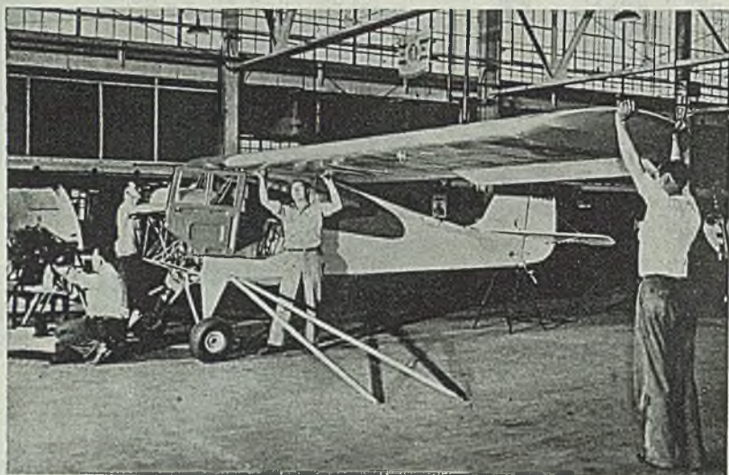
CIVILIAN PLANE: First Aeronca Champion postwar civilian airplane comes off the assembly line at Middletown, O. Plane is a tandem two-seater, has a cruising speed of 90 miles an hour, landing speed of 38 miles an hour, cruising range of 270 miles, and costs $2095. NEA photo
