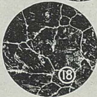
Fig. 17 — Fine grained steel as shown by McQuaid-Ehn test. Nitral etch. X100
