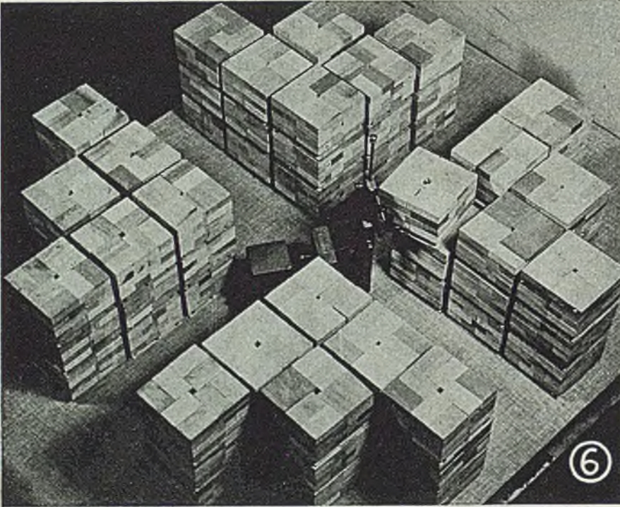
Fig. 9—BuOrd's 8-way 35 x 45½-in. pallet can be loaded into a freight car either two or three abreast, provided overlap is small. A wide range of loading patterns is possible. Photos Figs. 5-9 inclusive made with small models at the Navy's Materials Handling Laboratory, Hingham, Mass.
