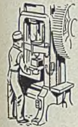
Plate samples are punched to rough form, then milled. Others are sawed, turned, drilled etc., as required.
