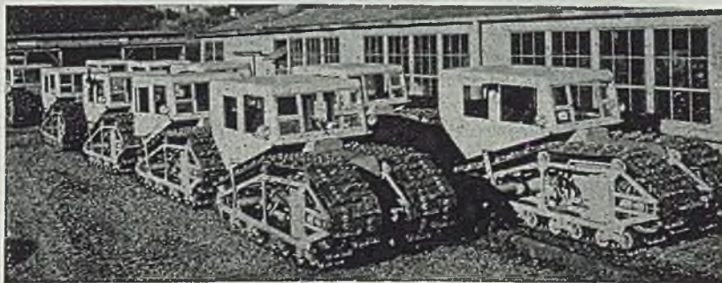
SNOW CRUISERS: Aluminum and steel construction of these tractors built by Iron Fireman Mfg. Co. of Portland, Oreg. allow them to be driven into large planes and carried to search areas for rescue, supply and scouting work of the Army Air Forces. The snow cruisers can be dismantled into four parts. Top speed is 18 miles per hour and maximum load over 2 tons. They will climb grades as steep as 35 degrees in deep snow, extra wide tracks and deep grousers aiding traction
