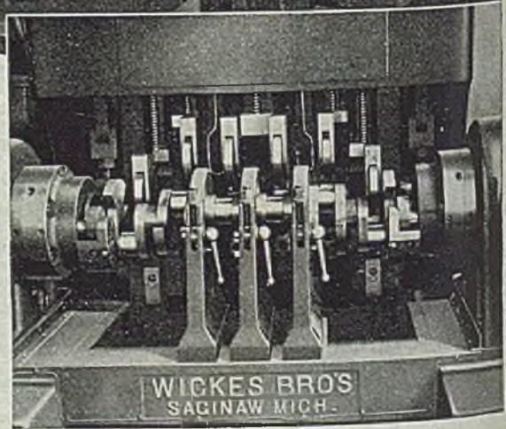
Inset shows tooling arranged for turning all crankpins on 6-throw aircraft crankshaft.
