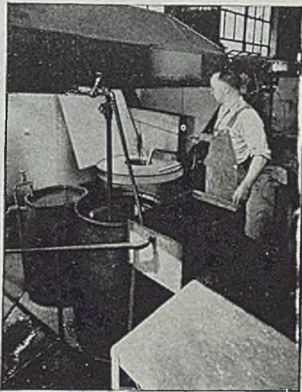
Salt bath hardening. Note nearness of quench tanks.
