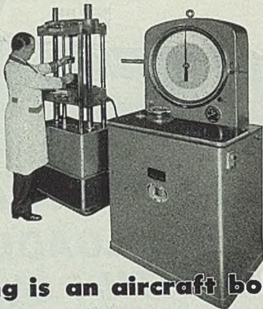
Aircraft bolts being tested on a Riehle P2 Precision Universal Hydraulic testing machine. Below—One of National Lock Co.'s nickel steel aircraft bolts.
