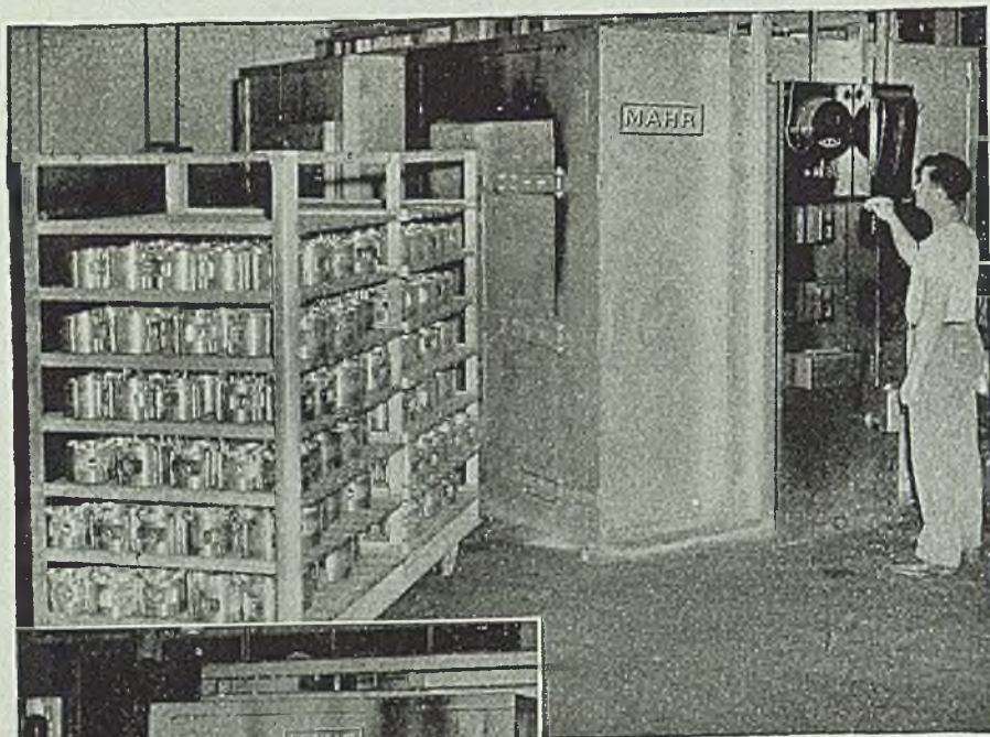
ABOVE: Strain-relief heat treatment of aluminum-alloy pistons before final machining, with MAHR electric oven.
