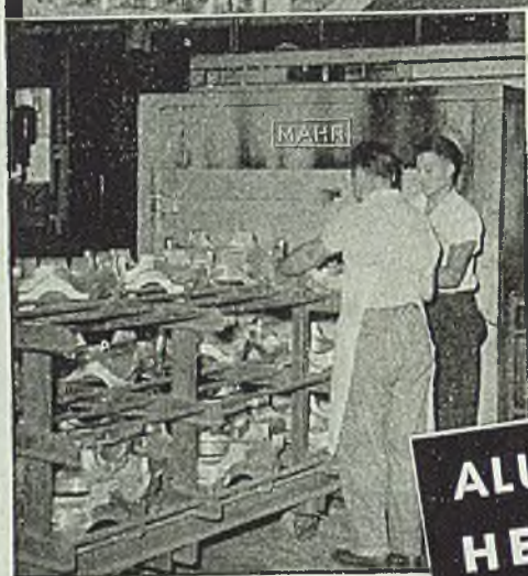
ABOVE: Strain-relief heat treatment of aluminum-alloy pistons before final machining, with MAHR electric oven.
