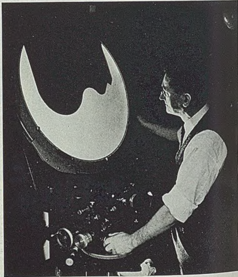
ULTRAFINE WORLD: Checking a thread gage smaller than a thumb nail is relatively simple when this comparator at Westinghouse Electric Corp. is used. By a system of mirrors, the gage, above, has been enlarged 100 times to facilitate study of its contours for absolute accuracy
