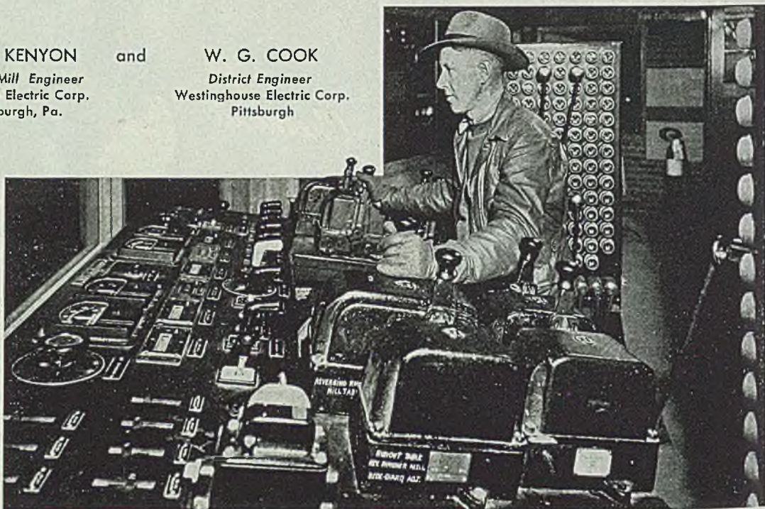
Fig. 1—Master control benchboard and preset pass selector plug boards for the reversing universal rougher
