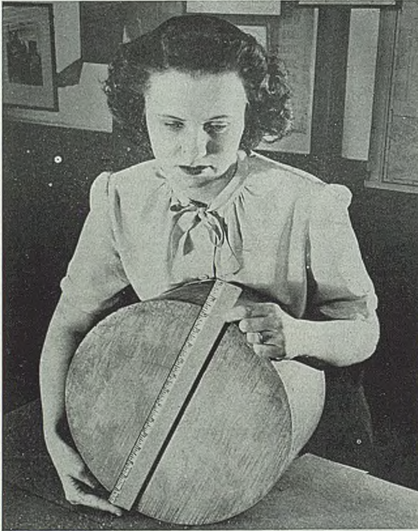
POWDERED METAL: Tipping the scale at 228.7 pounds, this piece of self-lubricating Oilite bronze bar stock made from powdered metals weighs about 85 pounds more than the largest piece previously made by Chrysler Corp.'s Amplex Division. The material will be machined into spherical bearings for dynameters on high torque aircraft engine test applications
