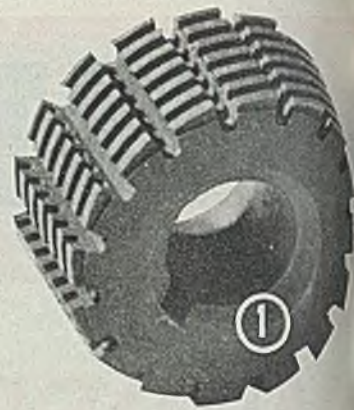
Fig. 2 shows a form-milling cutter, with clean, sharp edges, which was heat treated in the type TG furnace with a drycolene atmosphere. A square-thread milling cutter, heat treated in a TG furnace without decarburization or oxidation, is shown in Fig. 1. In Fig. 3, four types of cutters made of high-speed steels, heat treated in a type TG furnace with a protective atmosphere of drycolene, show a clean surface, but their cutting edges and corners are file-hard.
