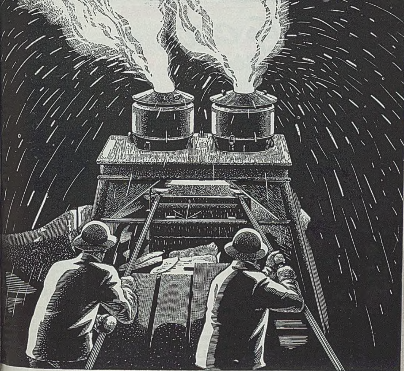
Pouring a double Thermit weld in fabricating a ship stern frame. ✓
