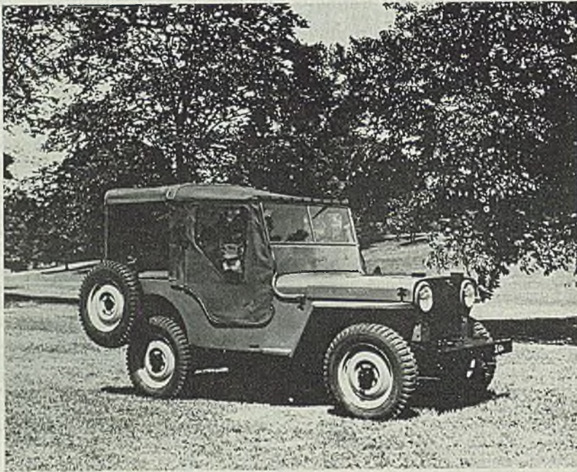
CIVILIAN JEEP: Combining the four basic functions of the tractor, light truck, mobile power unit and passenger conveyance, the postwar jeep is subject of an extensive promotion by the Willys-Overland Motors. The civilian model, recently unveiled, is equipped with removable top, front and rear. Willys is stressing its applications to farm tasks such as plowing, disking, mowing, raking, threshing, baling, sawing wood and similar jobs
