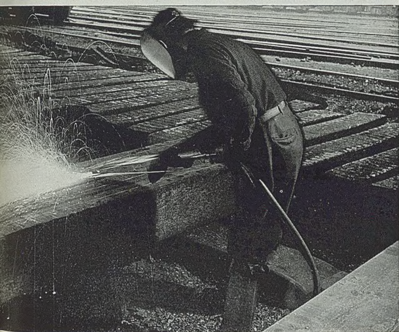
An Inland scarfer at work on a 12" x 12" bloom.
