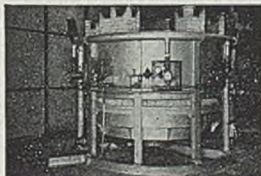
5'0" Size. Billet—2"x2"x14¾". Billets per hour—71. Pounds per hour—1190. Used with 1500 lb. hammer
