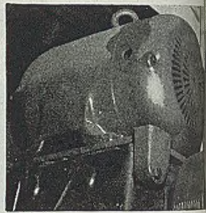
Century TEFC Motor mounted on a milling machine. Dirt on outside of fan cover is result of operation where air contains metallic dust and coolant spray.
