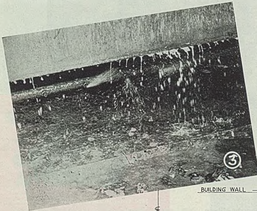
Fig. 3—This view through an open grating shows excess spray being removed by a water screen and flushed down an inclined apron into the water pit. Pit is cleaned three times a year
