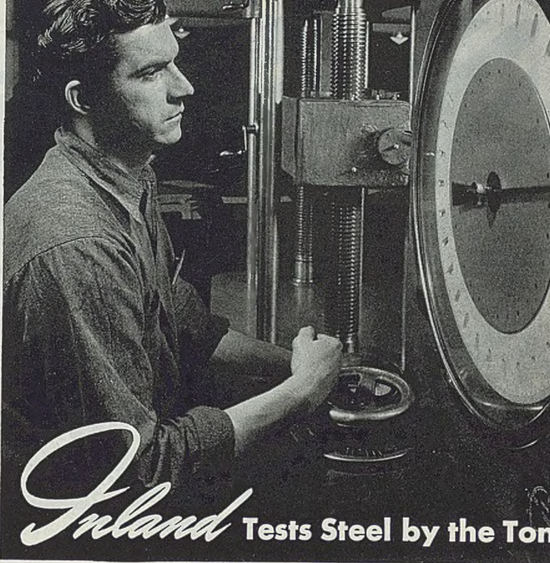
Operator determining physical properties on one of the many tensile testing machines in the Inland laboratory.
