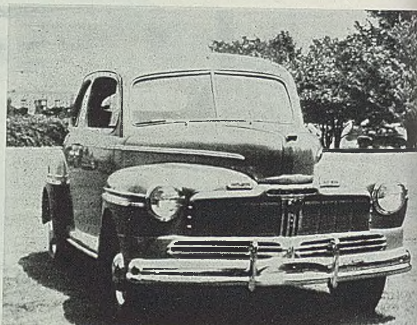
Handmade model of the new Mercury, to be produced by Ford within 60 to 90 days, reveals principally a redesigned front end, making extensive use of zinc die castings. First new Fords already are rolling from assembly lines. NEA photo
