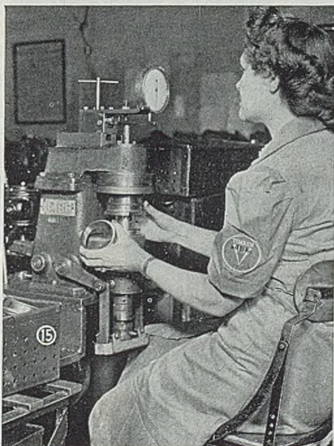
Fig. 12—Races are heated for hardening in rotary furnaces like the unit at right, then to avoid distortion are quenched in special dies in machines such as shown at left
