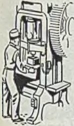
Plate samples are punched to rough form, then milled. Others are sawed, turned, drilled etc., as required.
