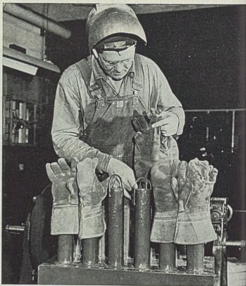
"INSULATING" WELDING GLOVES: Novel safety device at Graham-Paige Motors Corp., Detroit, is this mitt-dryer designed to protect employees welding amphibian tanks. Perspiration, with its high salt content, is a good conductor of electricity and increases the danger of serious shock to workers handling electrical equipment. To eliminate the hazard, welding gloves now are dried rapidly by slipping them over narrow chimneys protruding from a metal cabinet which contains a heater and fan
