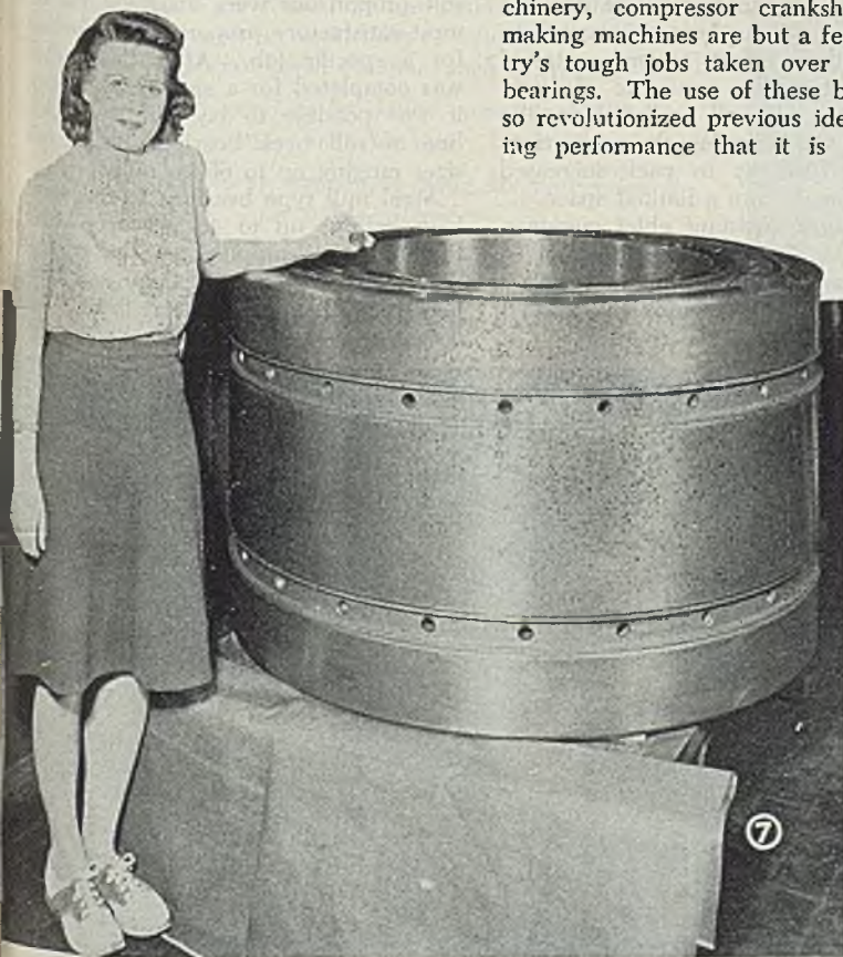
Fig. 4—Shoulders on inner race keep rollers positioned lengthwise so they divide the load equally, thus extending life
