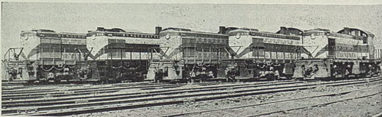
ALL DIESEL UNITS: These diesel-electric locomotives built by General Electric and American Locomotive Co. for the New York, Susquehanna & Western Railroad
