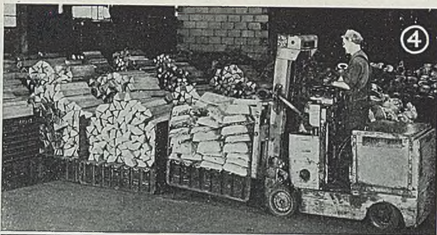
Fig. 4—Skid boxes from mold conveyor are picked up by fork truck and go to temporary storage for use in making up batches
