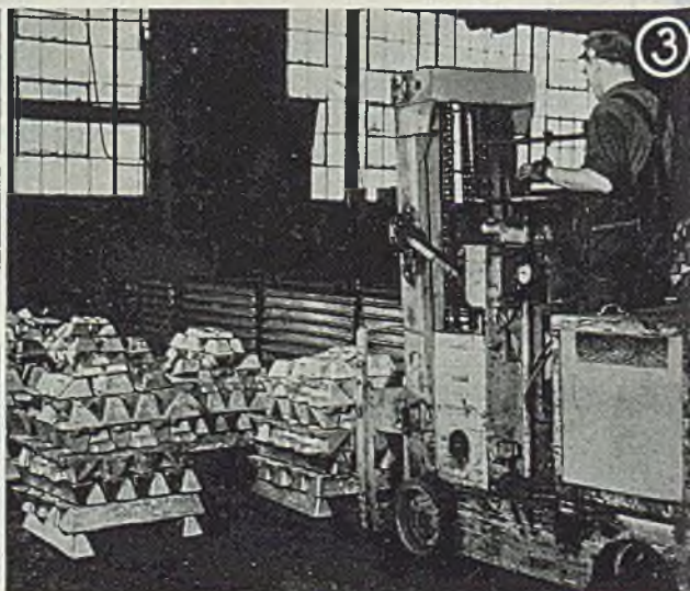
Fig. 3—Batches weighed are stacked temporarily using a pair of pigs in lieu of a skid
