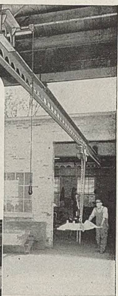
Left: Much time is saved because one man can pick up and deliver heavy parts with ease and safety. The equipment shown is hand propelled.
