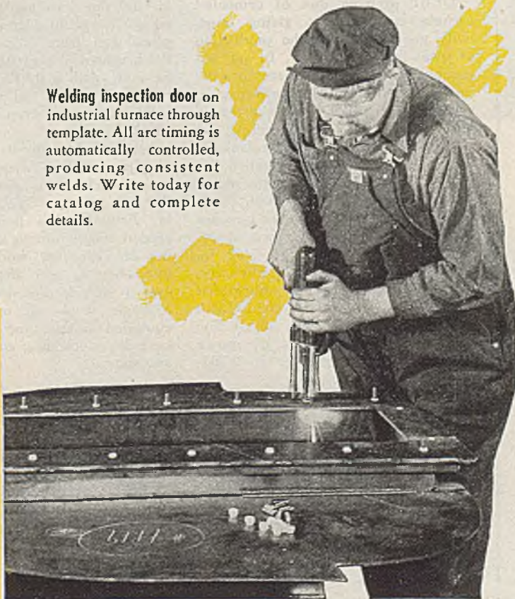
Welding inspection covers of all types is an ideal stud application. Studs are welded at desired centers to cover flange and cover secured with nuts. No holes in casing . . . close tolerances held.
