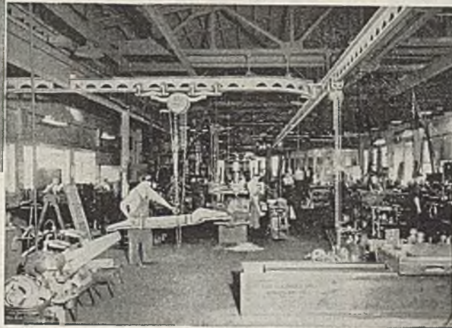
Left: Much time is saved because one man can pick up and deliver heavy parts with ease and safety. The equipment shown is hand propelled.
