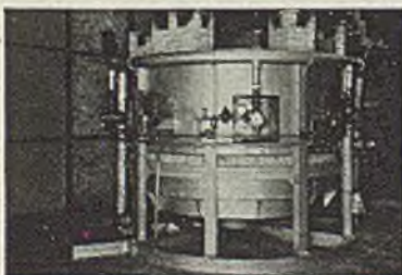
5'0" Size. Billet—2"x2"x14 \frac{3}{4} ". Billets per hour—71. Pounds per hour—1190. Used with 1500 lb. hammer
