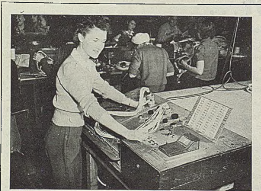
PINBALL MACHINE GOES TO WAR: Boeing Aircraft Co. production engineers are using part of the mechanism of a pinball machine to check automatically the continuity of B-29 wire connectors. Some of the Superfortress wiring harnesses contain as many as 52 separate wires which formerly were checked individually. This device permits speedier and more accurate tests
