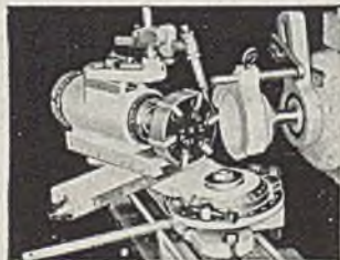
Grinding radius on 4" Insert Tooth Face Mill
