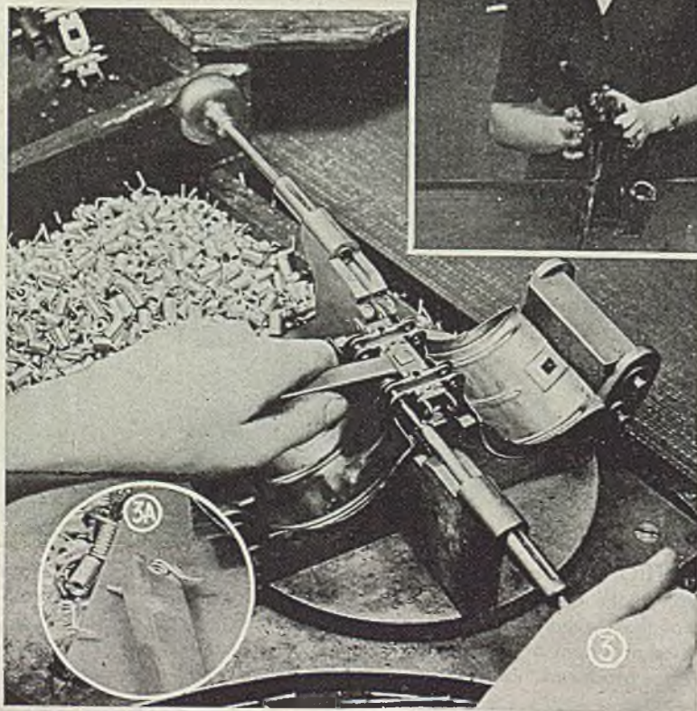
Fig. 2—Assembly line starts at rear; finishes in foreground where operators are locking hinge pins by flattening ends in revamped wire cutters. Parts travel down line on belt conveyor in center of table
