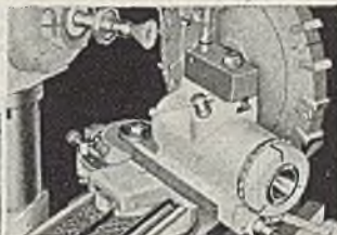
Grinding radius on a 10" Milling Cutter
