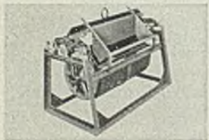
Loading stand with hopper.
