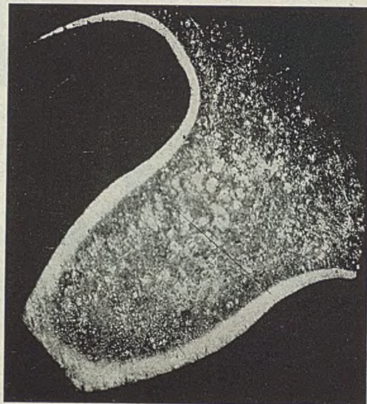
Cross section of SAE-4140 steel gear tooth, hardened by 5 megacycle 25-kilowatt induction heating equipment to a depth of 0.005-inch, with rockwell C hardness 58-60. Magnification about 10 diameters
