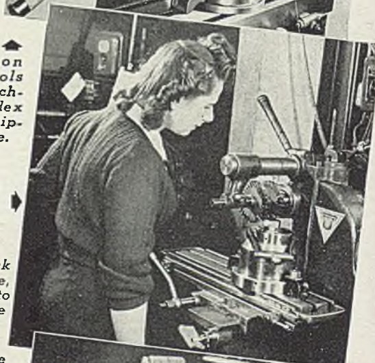
2" Zagar Index Fixture on a U. S. hand mill, milling hexes on bolts.
