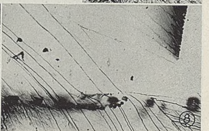
Fig. 12—Phase determination. Ordinary polished specimen of 18.10 per cent ferrosilicon etched with 25 per cent HNO_3 . X100
