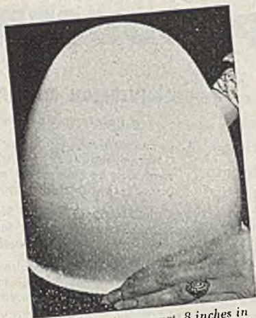
This deep drawn part, 8 inches in diameter by 7½ inches deep, was made from 18-gage Ti-Namel Steel and then given one coat of white enamel.
