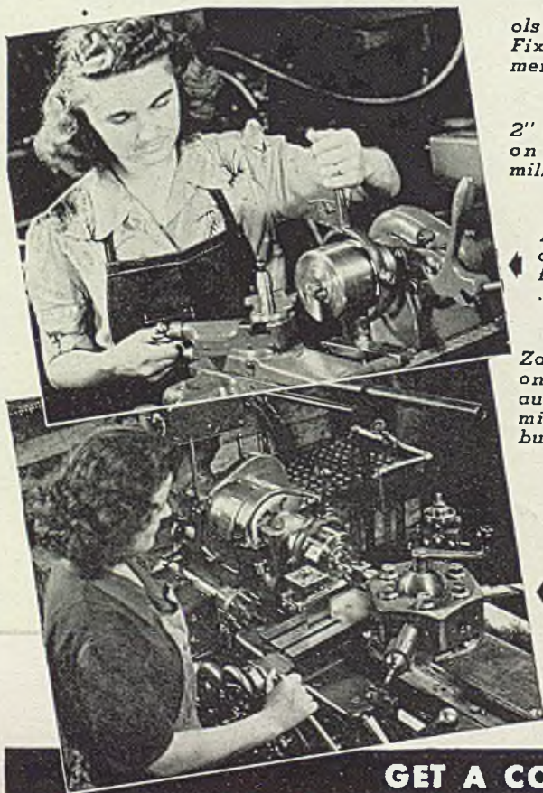
2" Zagar Collet Lathe Chuck on 16" South Bend turret lathe turning a job on which length dimensions and concentricity are all-important
