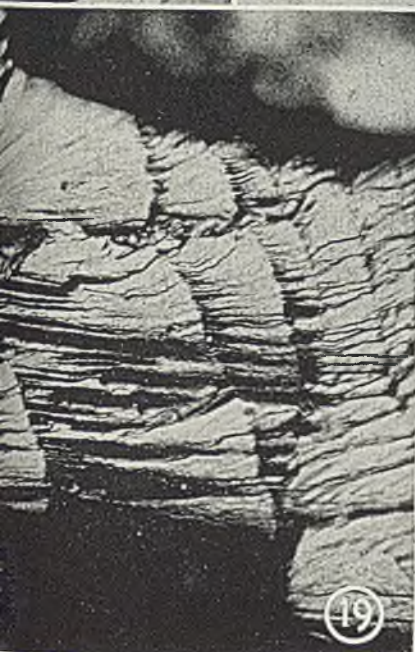
Fig. 11—Heat-etched fracture of specimen in Fig. 10. X500
