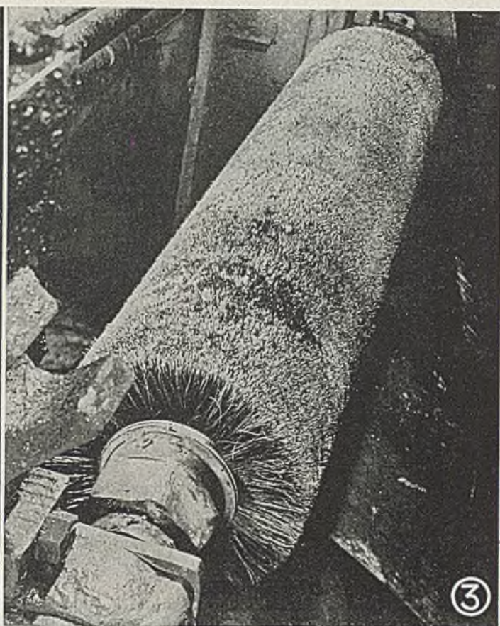
Figs. 1 - 3—These unusual photographs taken in a large midwestern steel mill show strip entering the scrubber of a continuous strip mill (Fig. 1) and leaving the scrubber (Fig. 2). In Fig. 3, a brush has just been installed and is ready for use
