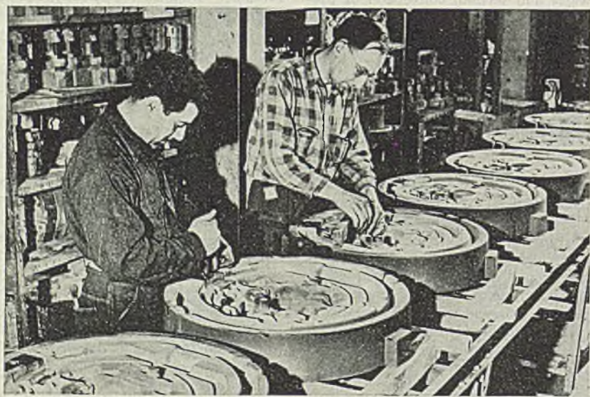
FOR LIGHTER AIRCRAFT: Increasing use of magnesium to lighten aircraft weight has enabled Superfortresses to carry added bomb loads against Japan. A core assembly operation, one of the important steps in casting the metal, is shown above in the plant of Bendix Aviation Corp.'s Eclipse-Pioneer foundries at Teterboro, N. J.
