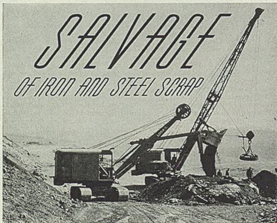
Power shovel and crane-operated magnet operate as a unit in the reclamation of metallics
