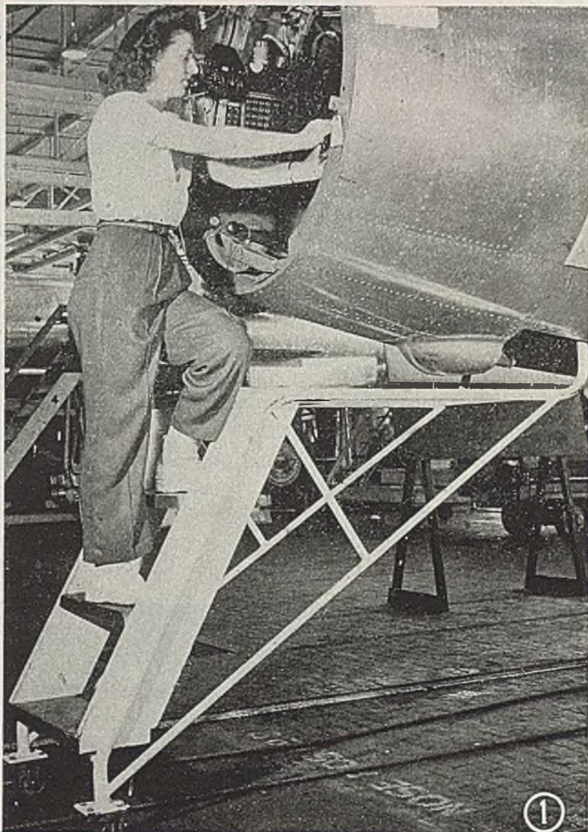
Fig. 1—Work on nose installation is facilitated by special ladder
