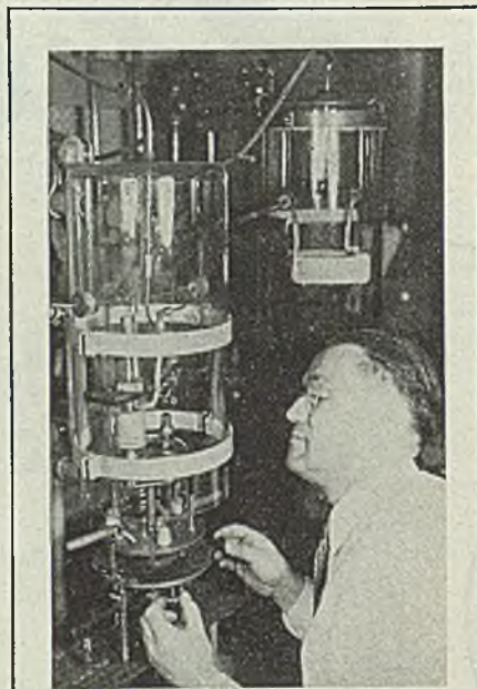
AIDS ELECTRONIC TUBE PRODUCTION: Anode and grid caps are sealed to bulb of 833A transmitter tube at Dobbs Ferry plant of North American Philips Co. Inc. High frequency coil heats metal by means of induction, and bell jar is filled with nitrogen to reduce oxidation of metal
