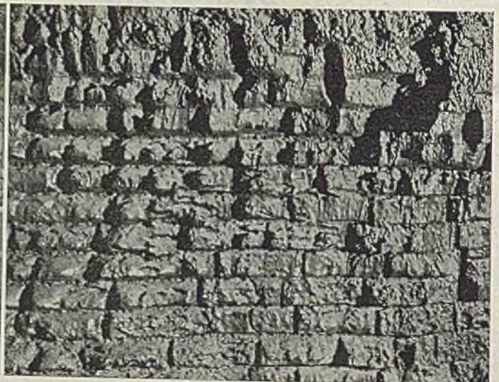
Fig. 3 (right)—Erosion of brickwork in a hot metal mixer
