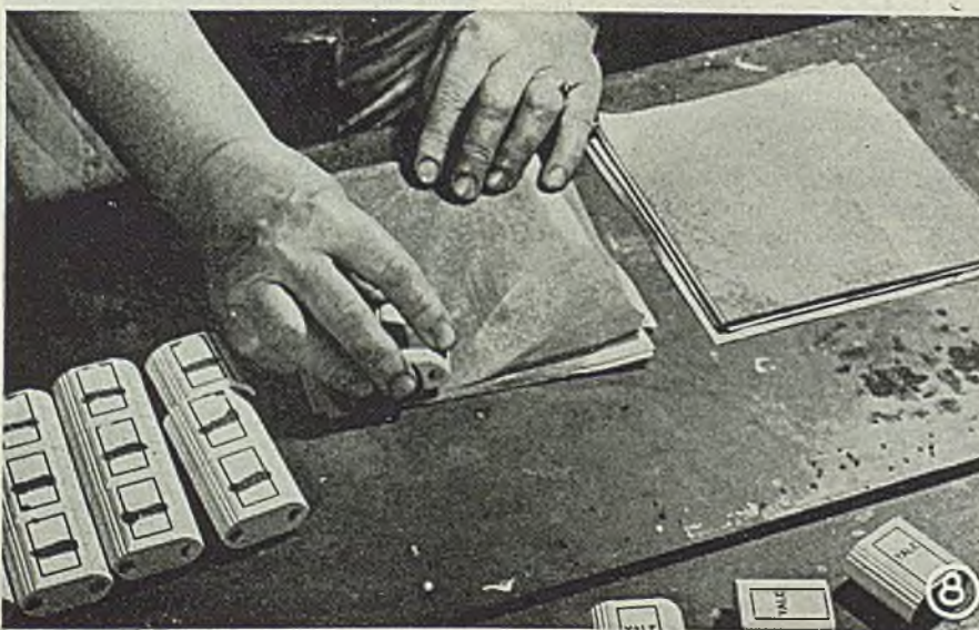
Fig. 8—Contrasting colored letters and decorative lines are wiped into padlock case after the finish has been applied to the depressed areas and dried in infra-red ovens
