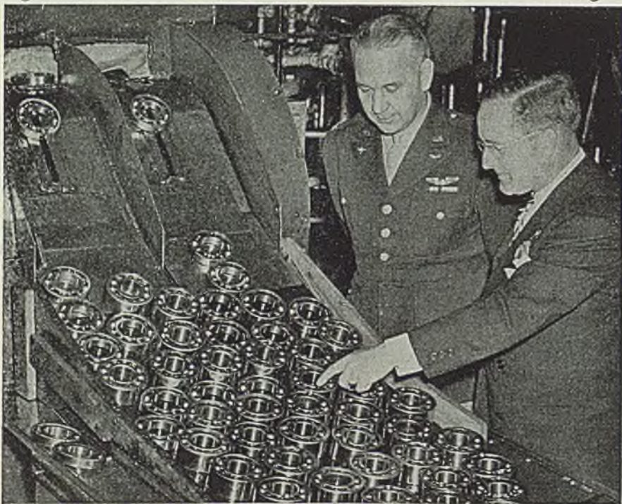
Ball bearings for the Packard-Merlin aircraft engine go through the final oil washing process at plant of Ahlberg Bearing Co., Chicago. Shown inspecting them are Colonel Finkenstaedt and Fred O. Burkholder, company president
