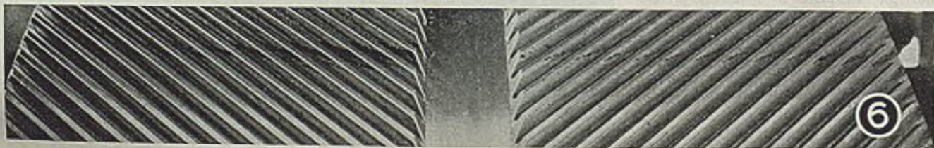
Fig. 6—Contact impression on gear after shaving
