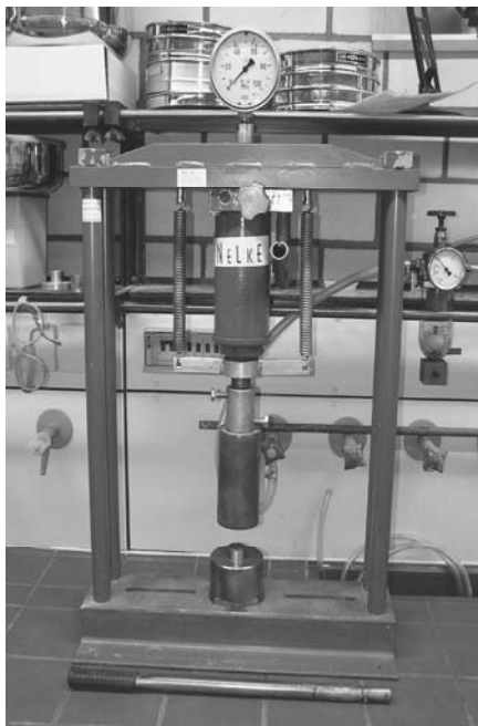
Fig. 1. The laboratory hydraulic press “Nelke” equipped with pressing form of inside diameter 30 mm
