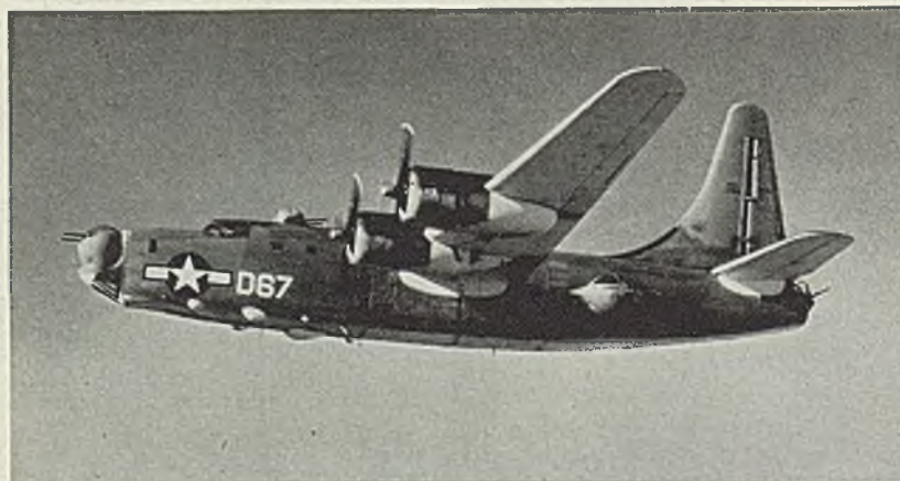
NEW NAVY DREADNAUGHT: The Privateer PB4Y-2 is the latest land-based patrol bomber built for the Navy by Consolidated Vultee Aircraft Corp., San Diego, Calif., which has orders for $40 million worth of the craft. The fuselage is 7 feet longer than the original B-24 Liberator. Top speed is 250 miles an hour, range more than 3000 miles, and gross weight varies from 62,000 to 65,000 pounds
