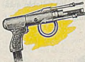
Complete fusion of studs to metal results from flux-filled studs, automatic timing control, and a full-shielding of the arc.
