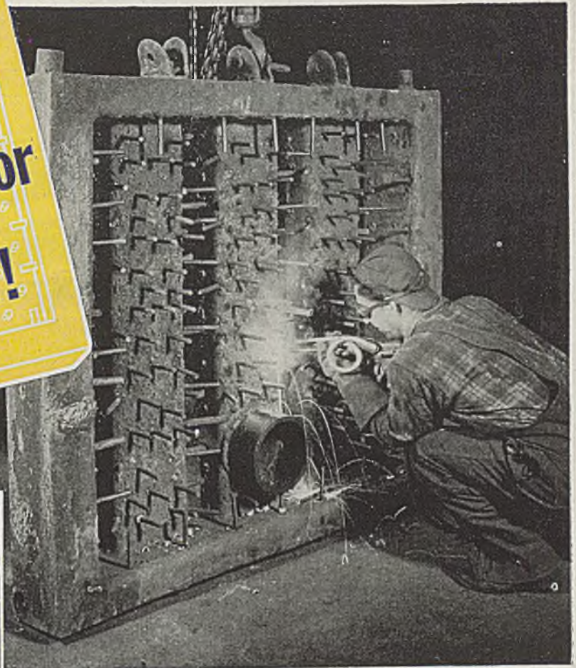
The Nelson Stud Welder automatically end-welds studs to metal. Photo at Inland Steel shows stud welding of a hearth door before installing refractory ore.
