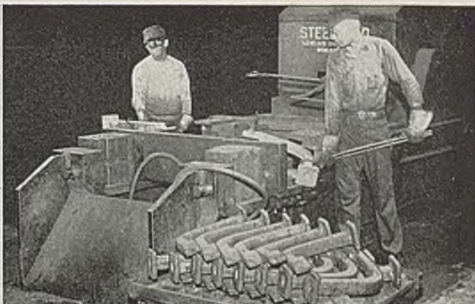
Truck braces made in three operations of .40 carbon steel 2 x 3 inch cross section bent to 5 1/2 inch inside radius on No. 6 Bulldozer.
